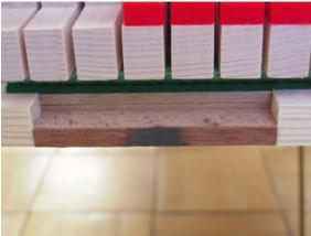
If most hammers are aligned towards the left from strings, glue a shim (wood veneer or thick paper) to the back side of Action Block.
