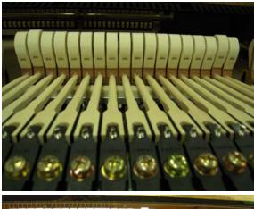
Level Hammers in each section using the capstan screws.
