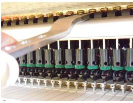
Adjust the left edge of hammer to be even with the left string. After all hammers are spaced even with the strings, remove the metal ruler from the action stop block.
