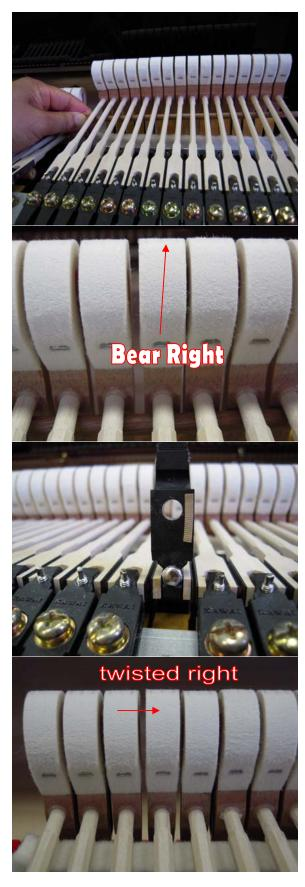
Checking hammer angle – spaces between hammers must be equal and parallel at the "rest" position.
