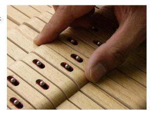
Ease any tight balance hole bushings with key easing pliers.
