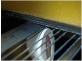
To move the action forward glue a shim (thin wood veneer) onto the hard wood block at the back side of the Keyframe. To move the action back, file the wood block. After the block is set correctly, then adjust the keyframe guides in the cheek blocks to match.
