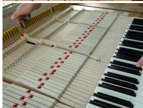
If the key sticks then ease the balance hole. This process must be done carefully until the key moves with the desired ease, but is not too loose.
