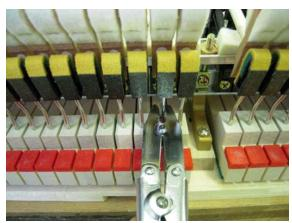
The backchecks must be uniformly spaced and their back surfaces parallel to the hammer line
