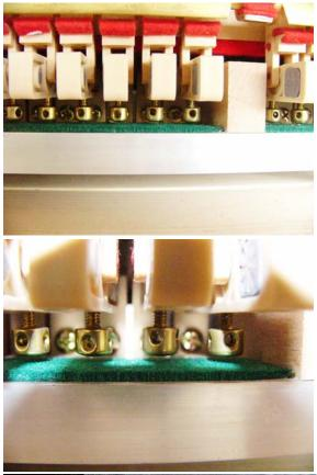
The head and pedal lever should be adjusted to create lost motion at the damper lever.
