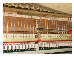
Adjust the lift height (sostenuto rod angle) with the capstan under the keybed. The sostenuto pedal should hold the dampers at the same height as the key.
