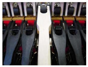
To adjust lateral position of the wippen, loosen the screw and shift the wippen over, or insert a piece of traveling paper behind the wippen flange on the side that you want the wippen to move towards.
