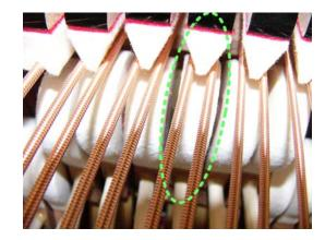
In the trichord note section the bass side of the hammer should overlap the left string 1mm.
