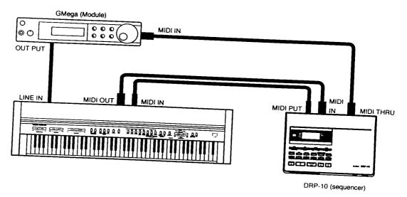
When connected as shown in the illustration, you can record songs played on the digital piano with the sequencer and play them back as many times as you like, and layer the module's tones made with the digital piano's MULTI TIMBRE function to assemble a complex automatic performance.
