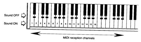
Use the 16 white keys at the left end of the keyboard to set the channels to ON. Use the 16 black keys at the left end of the keyboard to set the channels to OFF.
