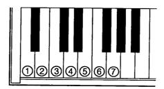
Volume is set to its lowest with the "1" key and at its highest with the "7" key. The "4" key is the factory setting.
