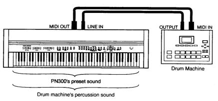
When connected as shown in the illustration, you can not only play along with the rhythm from the drum machine, you can also play the drum machine by striking the keys on the digital piano.
