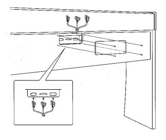
3. Connect the three cables to the connectors on the back of the speaker box. Make sure the connectors clicks in.
