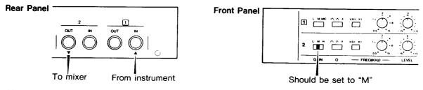
(2) Use the switches of ch1 and ch2 on the front panel to control the sound.
