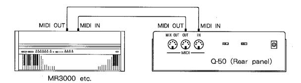
Use MIDI cables to connect the MIDI OUT of the digital piano to the MIDI IN of the Q-50 and connect the MIDI IN of the digital piano to the MIDI OUT of the Q-50.
