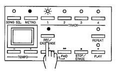
★While the REC/(EXCHANGE) button is lit, it is not possible to use the fast forward or rewind buttons, nor modify the time signature or tempo. To perform these operations, you must first press STOP/(ERASE) (■) and stop recording.
